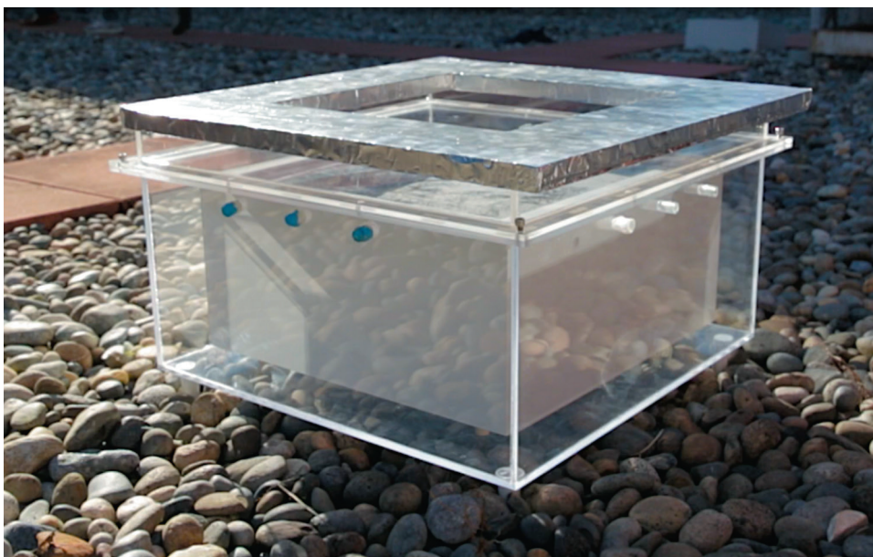
Figure 8: Second generation MOF water harvester tested in the Arizona desert. Box-in-a-box design capable of harvesting water from air with no energy input aside from ambient sunlight.
