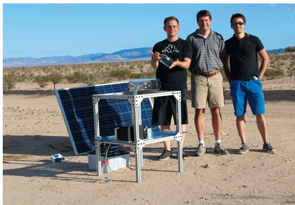
Figure 9: Third generation MOF water harvester tested in Mojave desert. It is powered by a solar panel to allow multiple cycles of water uptake from air and collection of water.
